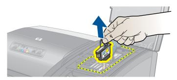
5 Install the new printhead in the color-coded slot that matches the color of the printhead.
